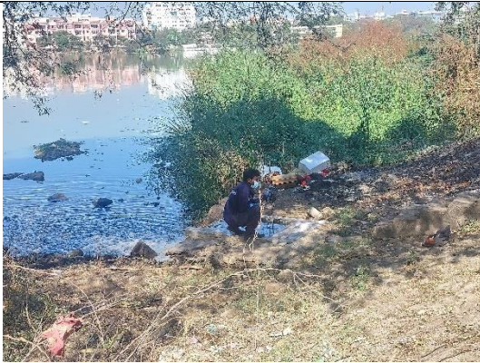
Figure 5: This image shows Point 3 demarcated on Figure 1 (Identified as the STP Outlet). Single Point measurement was collected on an hourly basis
