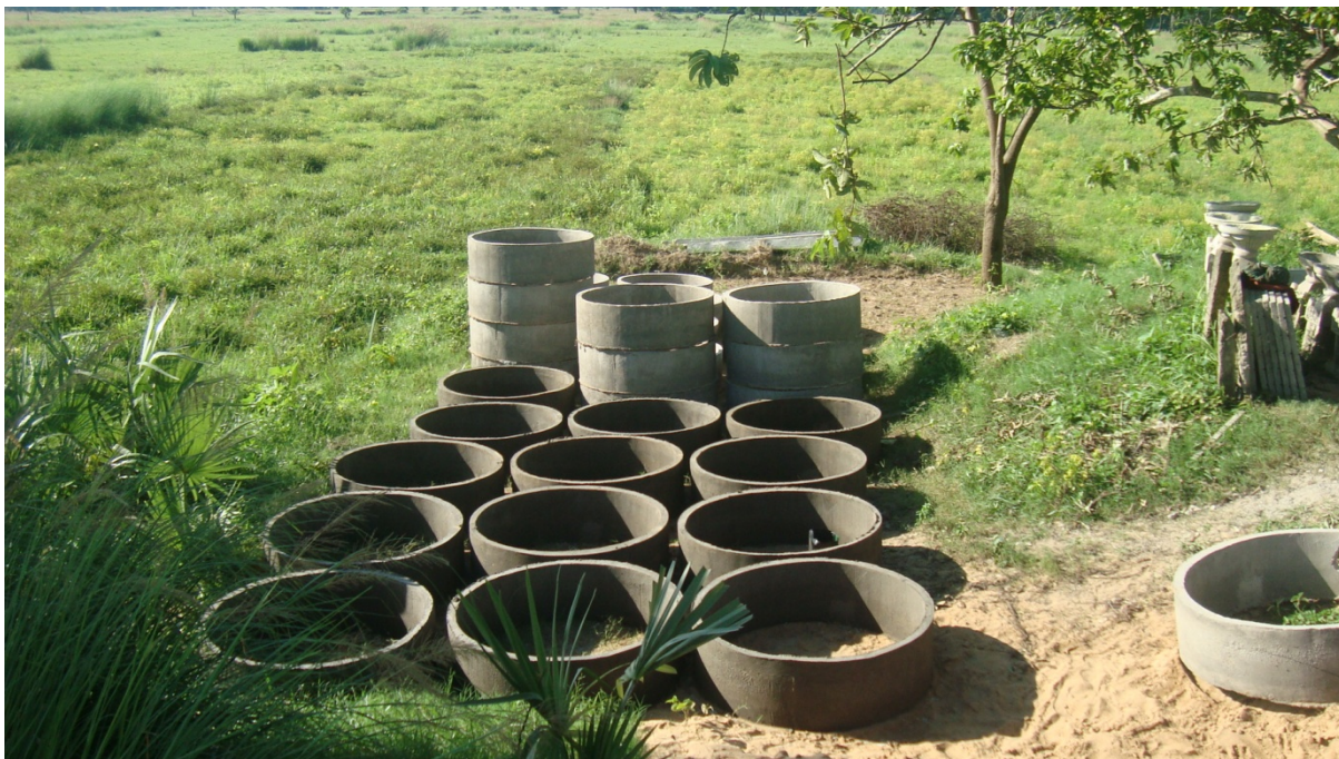
Figure 4: The rings made by masons to construct pit latrines made by Parmananda's Rural Sanitary Product Center
