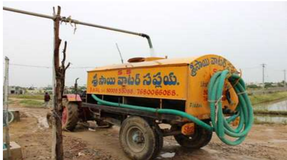
A 5500 litre tanker being filled from a private bore well in Kokapet
